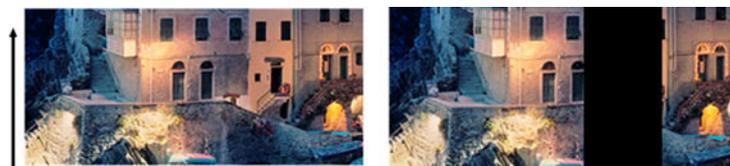
Original Scan affected by a failing scanbar
