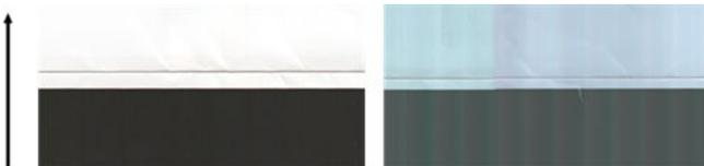
1. First, restart the printer and re-scan or copy. Clean and calibrate the scanner as indicated in [Clean the scanner scanbars on page 91](#) and [Calibrate the scanner on page 93](#). If the calibration failed, proceed as stated in [Calibrate the scanner on page 93](#). However, if the calibration ended correctly, scan your original again and check that the colored vertical bands have disappeared.
