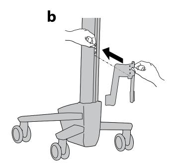
Note: Do not release t-nut until the bracket is completely in place or it may slide into the base of the cart.
